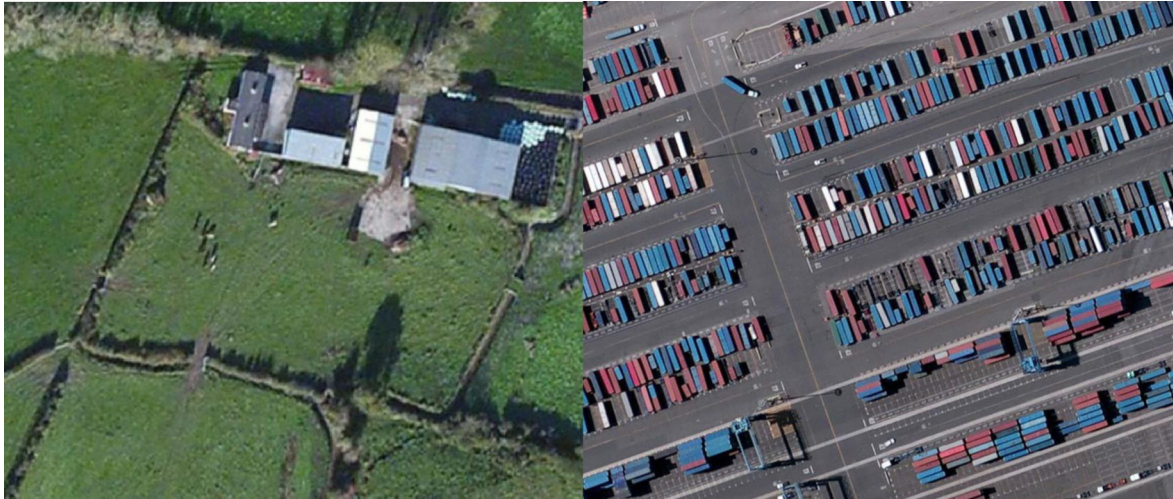
Figure 6.6.1 The level of detail of images available in many locations. In the first panel, horses can be seen grazing in front of the farm house, and hay bales can be seen wrapped and stacked to the right of the barn. In the second panel, the uniform grey of concrete, as well as individual containers and the cranes used to move them can be seen. Shape, size, texture and colour are important characteristics for identifying human threats on the environment.
