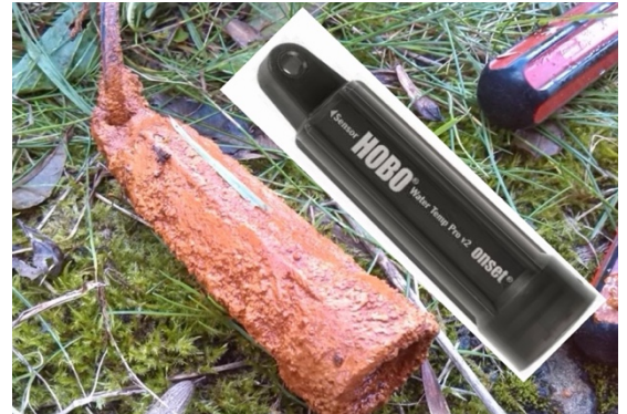
Figure 2.6 – Iron oxide deposition on temperature gauge used in South Wales mine water energy development site after 4 months of use compared to new temperature gauge. Source – Farr & Tucker 2015
