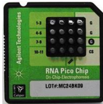
Fig. 3.5: RNA Pico-Chip. The chip accommodates sample wells, gel wells and a well for an external standard (ladder). Micro-channels are fabricated in glass to create interconnected networks among these wells. During the chip preparation, the micro-channels are filled with a sieving polymer and fluorescence dye. Once the wells and channels are filled, the chip becomes an integrated electrical circuit. The 16-pin electrodes of the cartridge are arranged so that they fit into the wells of the chip. Each electrode is connected to an independent power supply that provides control and flexibility (Agilent Technologies, 2008).
