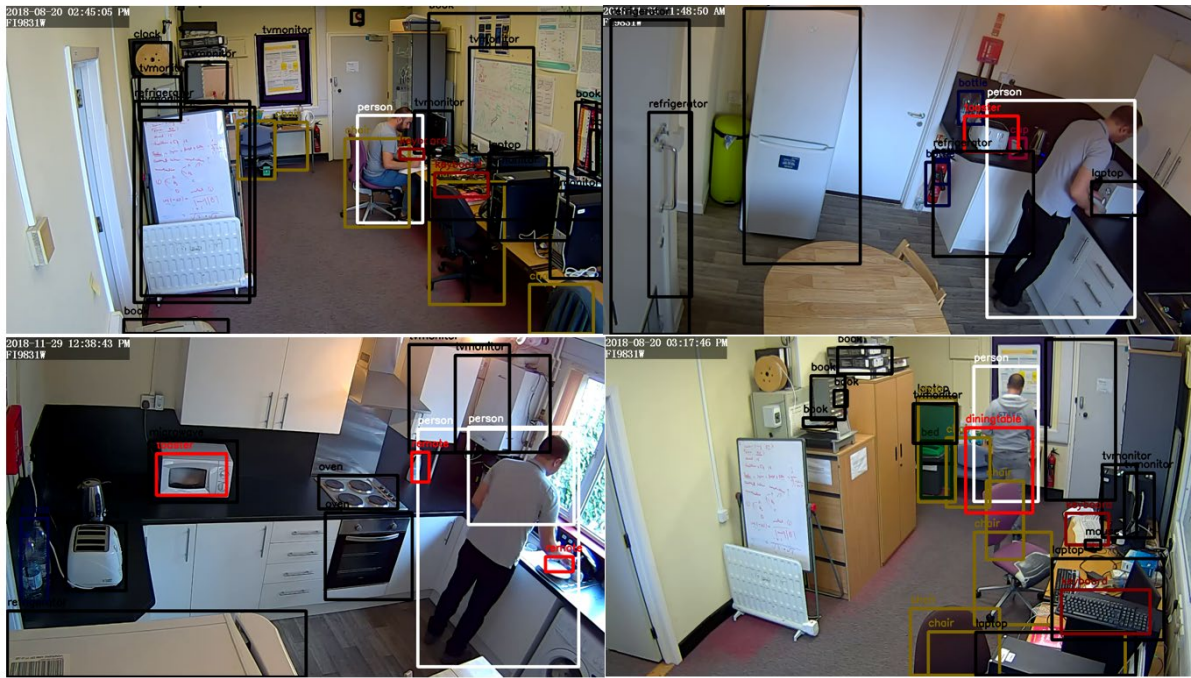
Figure 7. 1 Object detection using CNN (YOLO9000)
