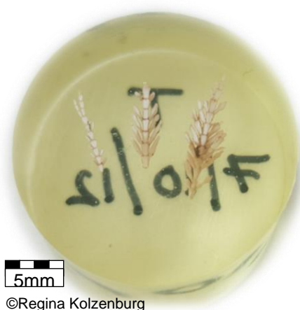
Figure 2.12: Example of embedded C. officinalis in Epoxy resin
