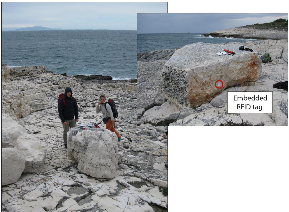
Figure 5.26. Tagged boulder on sloping shore platform; inset, tagged boulder, RFID tag circled. (Premantura, Croatia).
