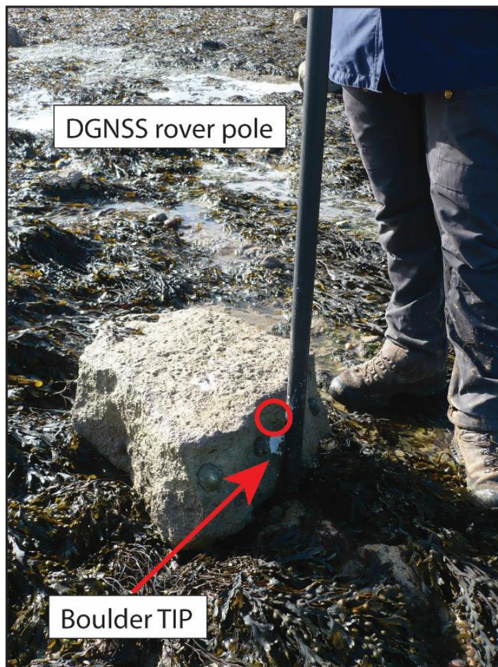
Figure 2.7. Recording of the boulder location; the DGNSS pole is positioned against the tag insertion point (TIP). The orientation hole is highlighted by the circle and the attached limpets are noted for purposes as described in Table 2.5, item 4.
