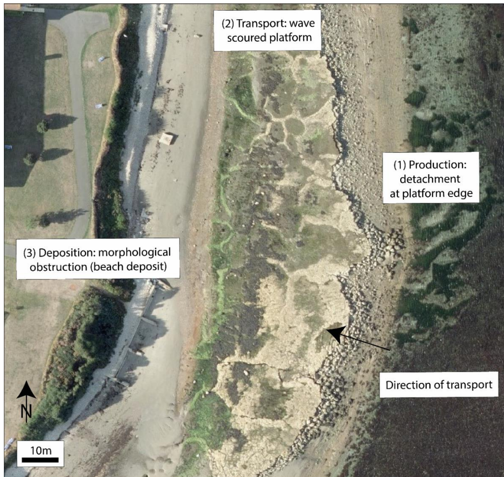
Figure 5.19. Shore platform edge at Bembridge Ledge - boulder production, transport and deposition. (Aerial image, Channel Coast Observatory, 2017b).
