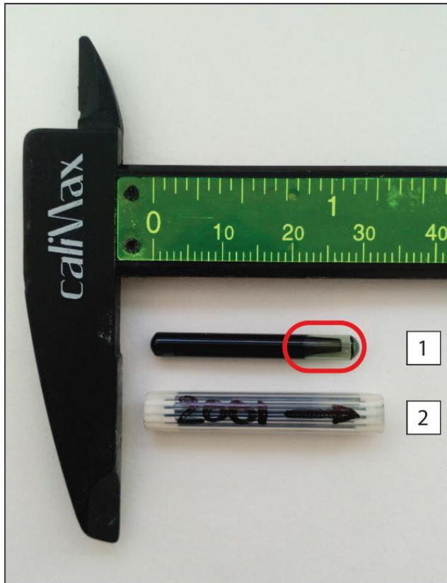
Figure 2.5. RFID tag; (1) 32 mm RFID tag, the copper coils are located in the transparent end of the tag, circled; (2) RFID tag within a numbered protective silicone sleeve.
