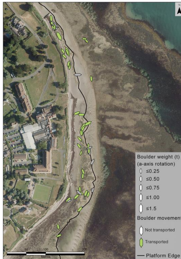
Figure 10. Bembridge Ledge site map identifying tagged boulder location, mass range, a-axis orientation and transport capacity. [Colour figure can be viewed at wileyonlinelibrary.com ]
