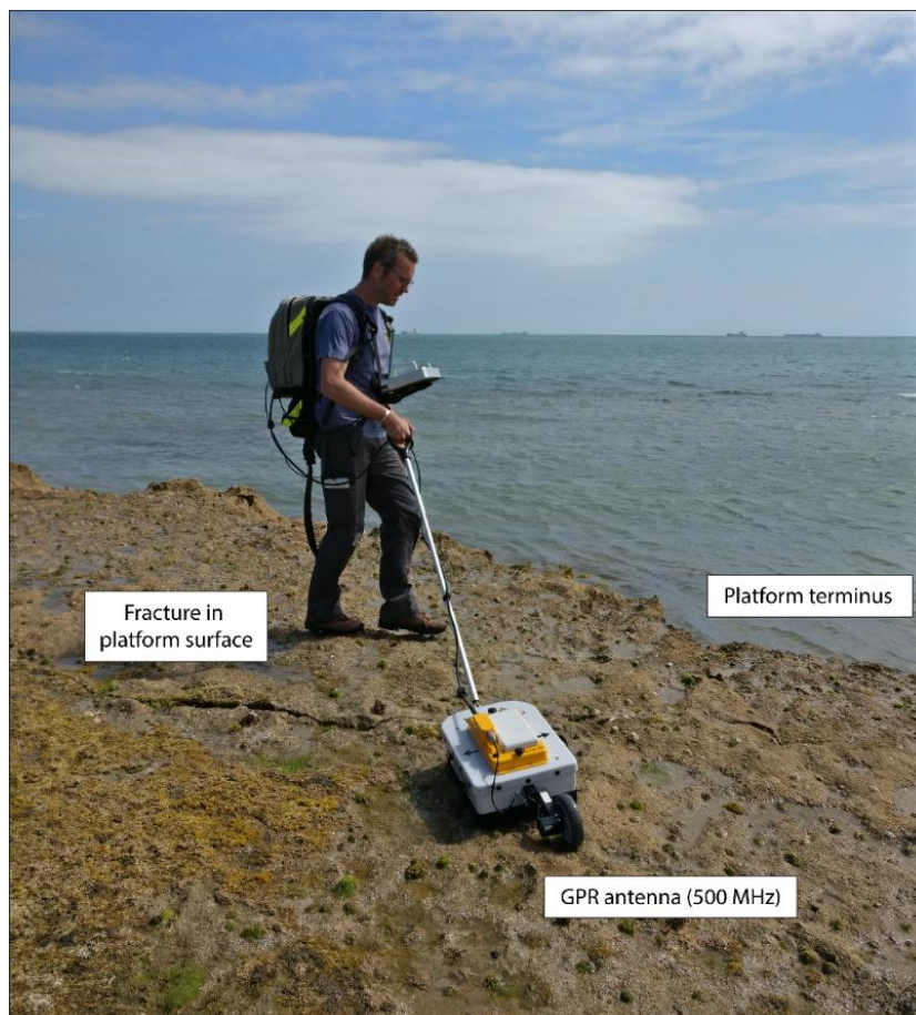
Figure 5.2. Mala GPR ProEx system with shielded 500 MHz antenna.
