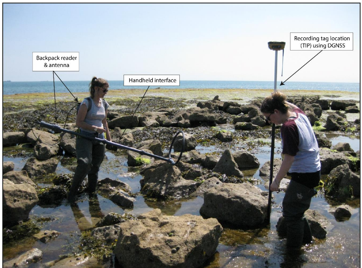
Figure 3.7. RFID tagged boulder relocation at BR using tag detection equipment (at left) and recording of boulder location using DGNSS (at right). For scale, the DGNSS pole is extended to a height of 2.0 m.
