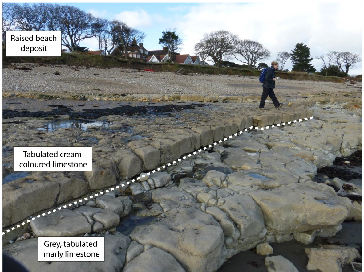
Figure 1.15. Subfacies of the Bembridge Limestone, heavily jointed limestone overlying marl-rich limestone, image from Bembridge Ledge.
