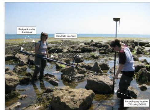
Figure 7. RFID tagged boulder relocation at BR using tag detection equipment (left) and recording of boulder location using DGNSS (right). For scale, the DGNSS pole is extended to a height of 2.0 m. [Colour figure can be viewed at wileyonlinelibrary.com]
