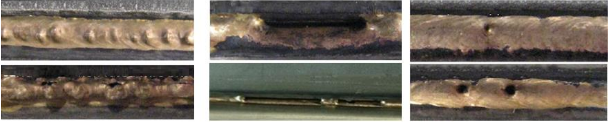
Figure 1.13 Different type of seam imperfections in the laser brazing process [30].
