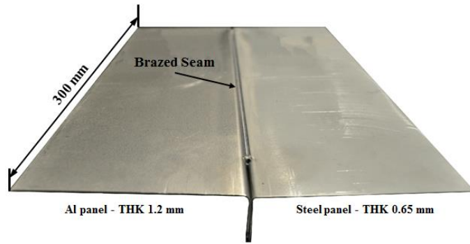
Figure 2.1 Laser welded-brazed coupon in coach peel configuration.
