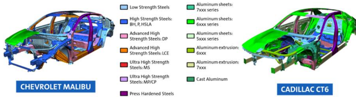
Figure 1.7 General Motors' first completed vehicle with a body made from mixed materials [16].
