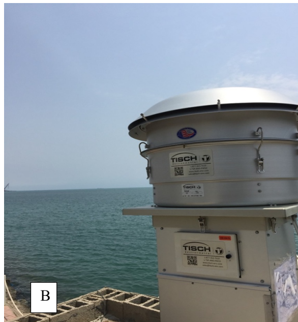
Figure 1. 3 Images (A) and (B) show the high volume air sampler near to the sea.
