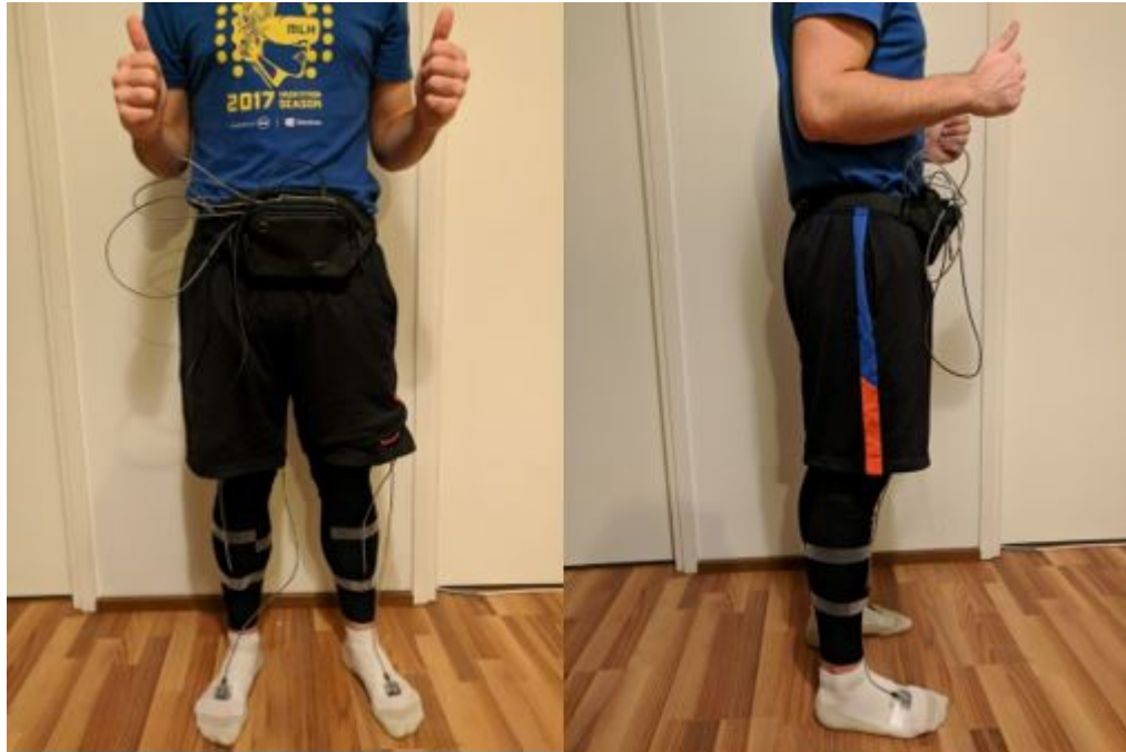
Figure 2. Subject wearing the sensor system, the Raspberry Pi computer is inside the hip pouch and the sensors are attached to the shanks and feet, tape is used to secure the sensors and their cables.
