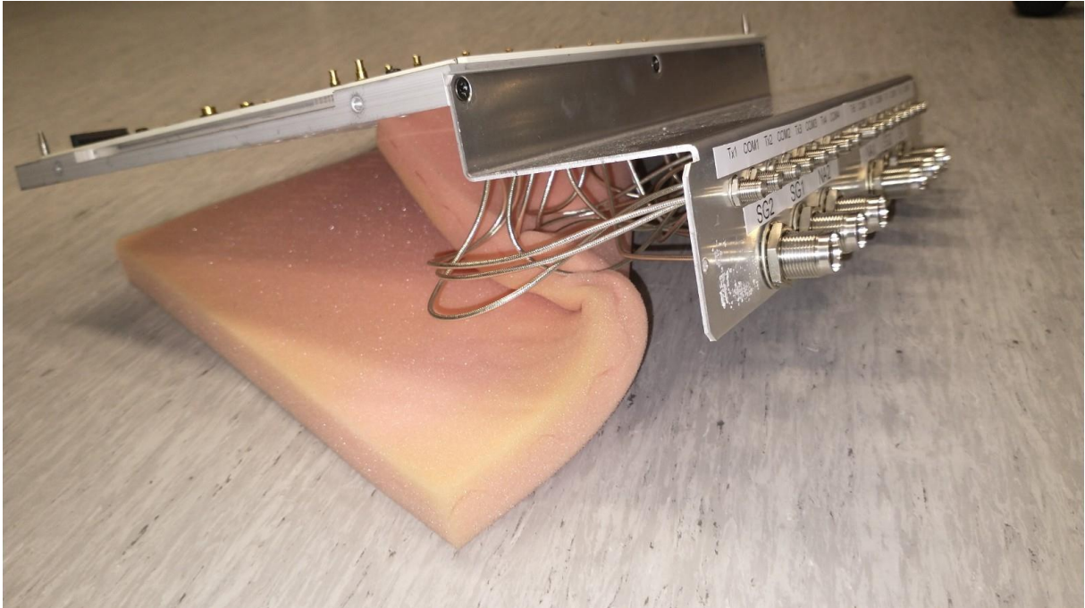
Figure 20. RF tester module assembled for calibration.
