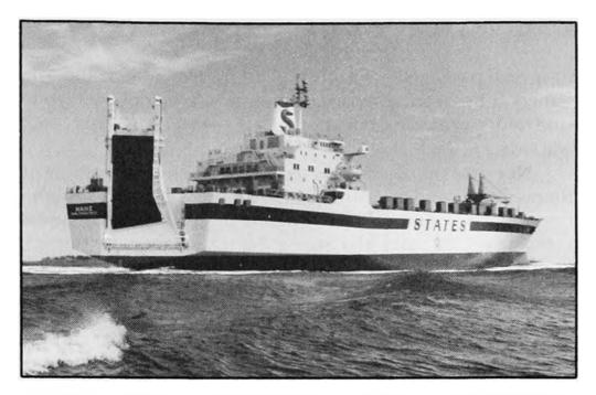
The Bath Iron Works "Ro-Ro" *Maine* is the lead ship in a class of four such vessels. The freighter, built with a large stern ramp to service ports with underdeveloped facilities all over the world, was launched in late 1975. Courtesy Bath Iron Works.
