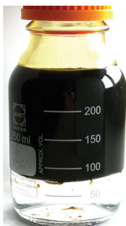
Figure 6. TDO oil, showing phase separation between organic oil and water layers. Reproduced from Case et al. (2012). 23
