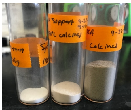
Figure 34. Comparison of dried ASA support, calcined support, and synthesized 20 wt% Ni/ASA catalyst.
