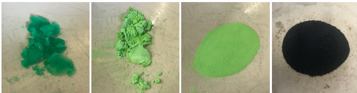
Figure 31. Stages of incipient wetness impregnation for a 20 wt% Ni/SiO 2 catalyst: 1) metal solution is added dropwise to the support 2) catalyst is dried in oven overnight at 100°C, 3) catalyst is crushed and prepared for calcination, 4) catalyst is calcined at 450°C for 3 hours.
