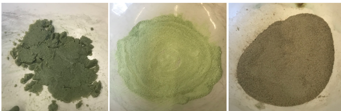
Figure 33. Various stages of incipient wetness impregnation using nickel on amorphous silica-alumina (ASA).
