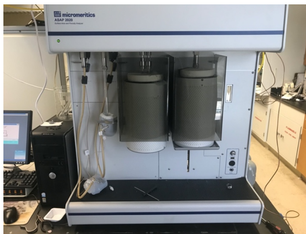
Figure 14. Micromeritics ASAP 2020 instrument used for nitrogen physisorption.
