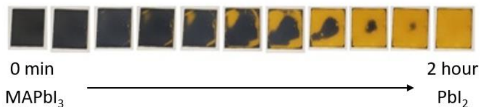
Figure 2.1 Pictures of \text{MAPbI}_3 sample degradation process under 150\text{ }^\circ\text{C} heating
