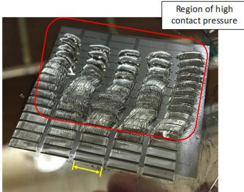
Figure 4.17 Feature distortion during inclined lithography. Scale bar = 6.39 mm
