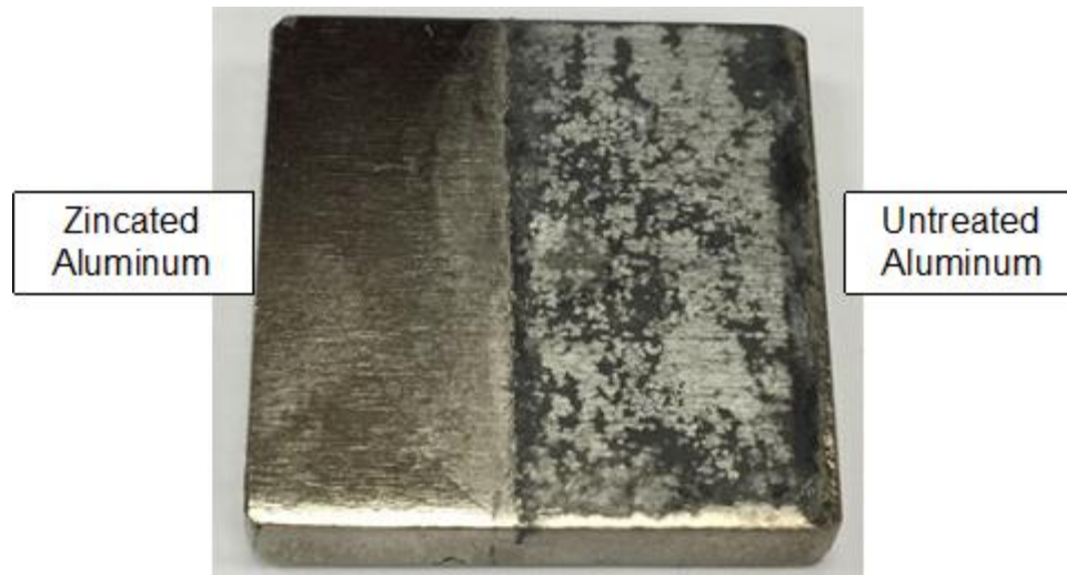
Figure 5.5 Effect of plating on zincated vs untreated aluminum surfaces
