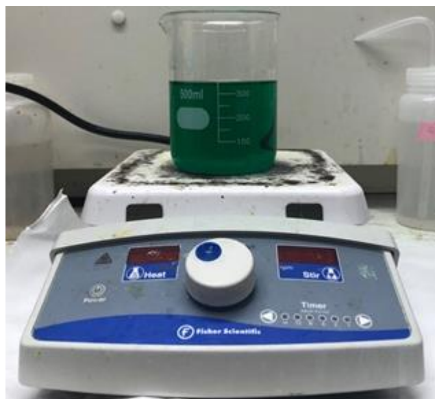
Figure 5.12 ENP solution setup on hot plate under fume hood
