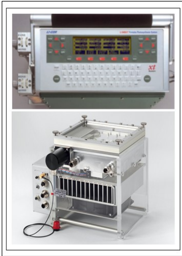
Figure S1 A photo of a LI-6400XT portable gas exchange system (top) and Walz 3010-GWK1 chamber (bottom) used in quantification of short-term temperature-response curves of R_{\text{dark}} and A_n in new-developed (ND) leaves. Airline tubes were used to connect the Walz 3010-GWK1 chamber to the LICOR Infrared gas analyser head with a water trap in between to remove excess humidity. Photos are courtesy of www.licor.com and www.walz.com .
