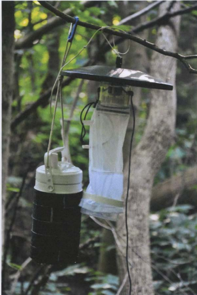
Figure 4. CDC light trap for collection of mosquitoes. The canister (left) was filled with dry ice which attracted mosquitoes into the motor driven trap (right). Traps were laid out between 15:00 and 09:00 hours.
