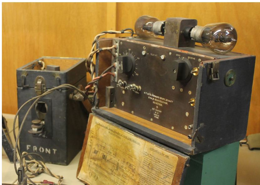
The transmitter and receiver of a Rear Station Mk II Wireless Telegraph Set Forward Spark 20 watt B ("Loop Set"). [Joe Costello, RCSigs.ca ]
