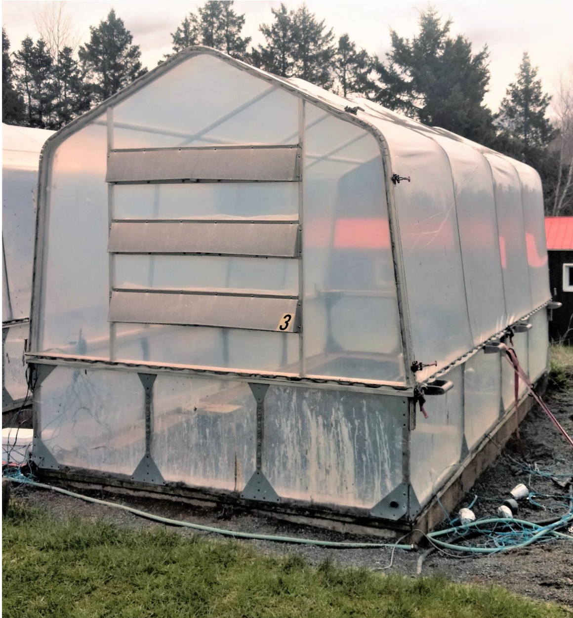
Image 2 Front view of in-ground, meso-scale manure tanks with continuously flow-through, steady-state chamber. Showing ambient air inflow vents.
