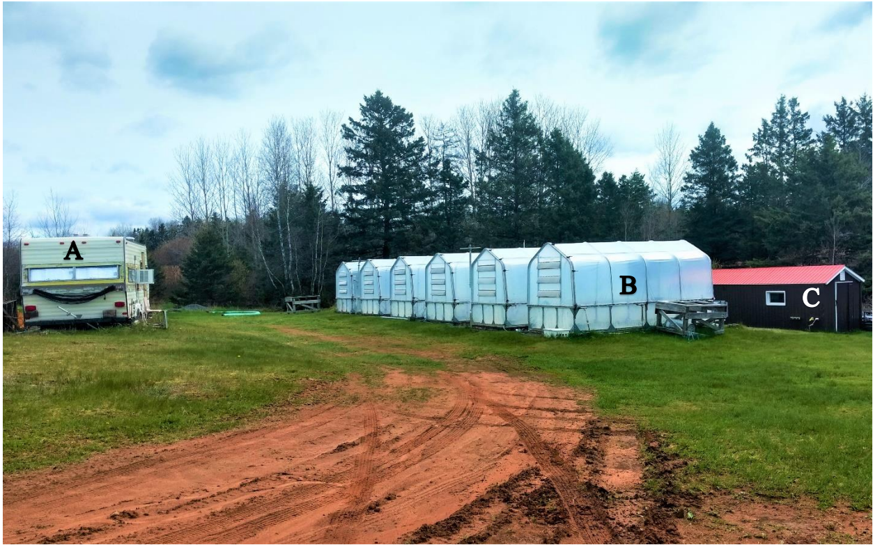
Image 1 Dalhousie University Bio-Environmental Engineering Centre experimental research site, showing instrument trailer (A) housing trace gas analysers, in-ground meso-scale manure with continuously flow-through, steady state chambers (B), and an instrument hut housing ammonia acid traps (C).
