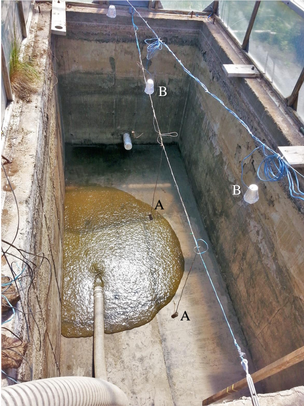
Image 4 Experimental manure tank during tank filling showing 80 cm depth manure thermocouples (A) and 10 cm above manure surface shielded air temperature thermocouples (B).
