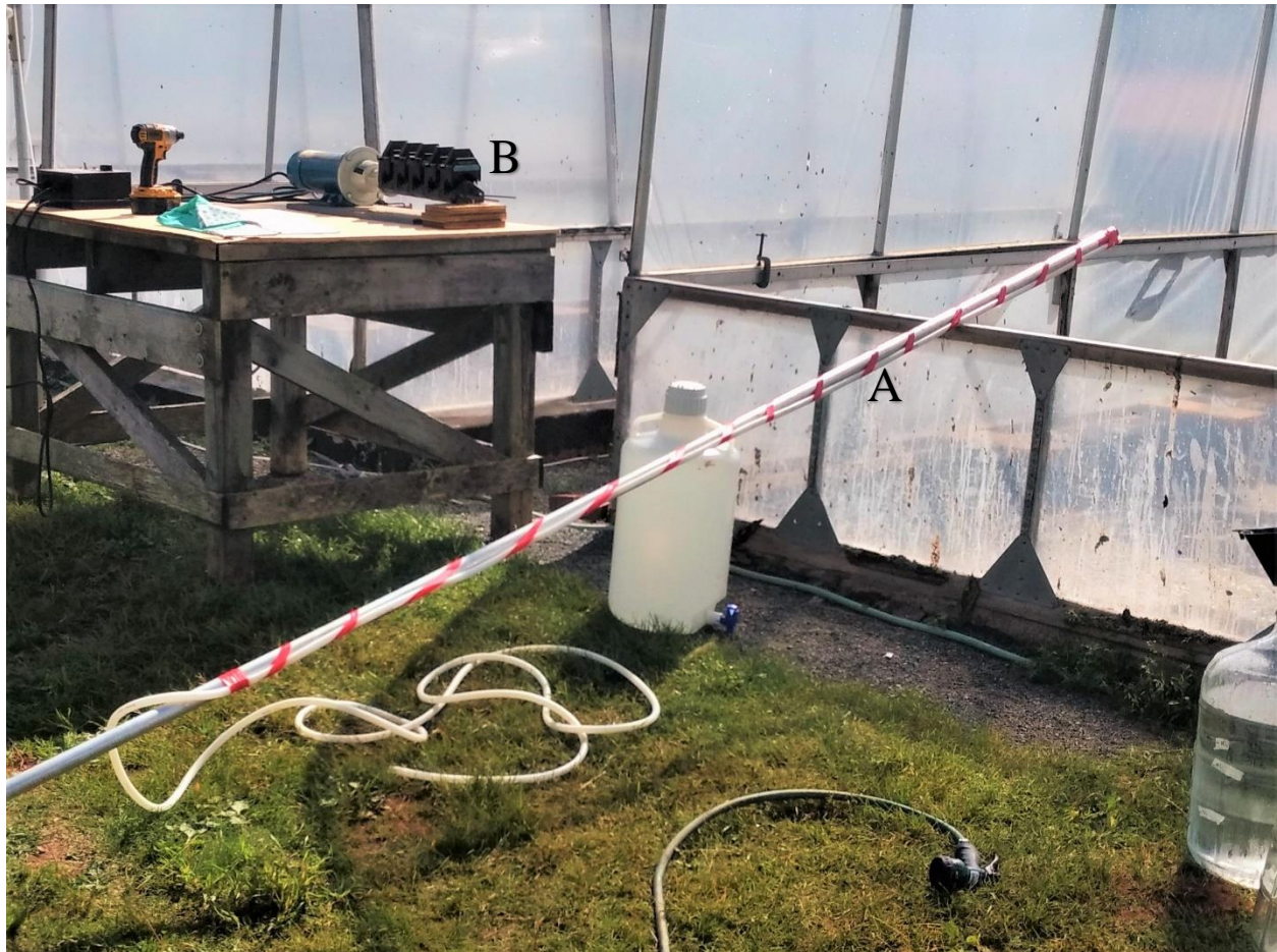
Image 5 Aluminium pole with acid resistant tubing taped to it (A) used for transferring sulphuric acid ( \text{H}_2\text{SO}_4 ) throughout the stored manure and a peristaltic pump (B).
