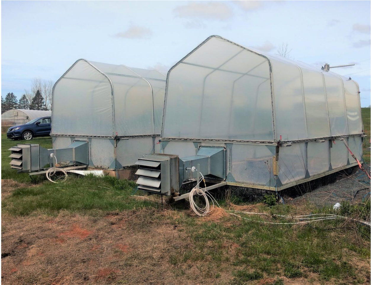
Image 3 Rear view of in-ground, meso-scale manure tanks with continuously flow-through, steady-state chambers attached. Showing the outflow vent with sample tubing.
