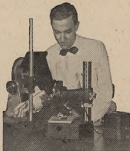
R. E. Suggs, B.S. in M.E., George Washington University, 1948, doing mechanical research to improve machine design. His optical-slit microscope measures surface scratches as fine as 20 millionths of an inch.
