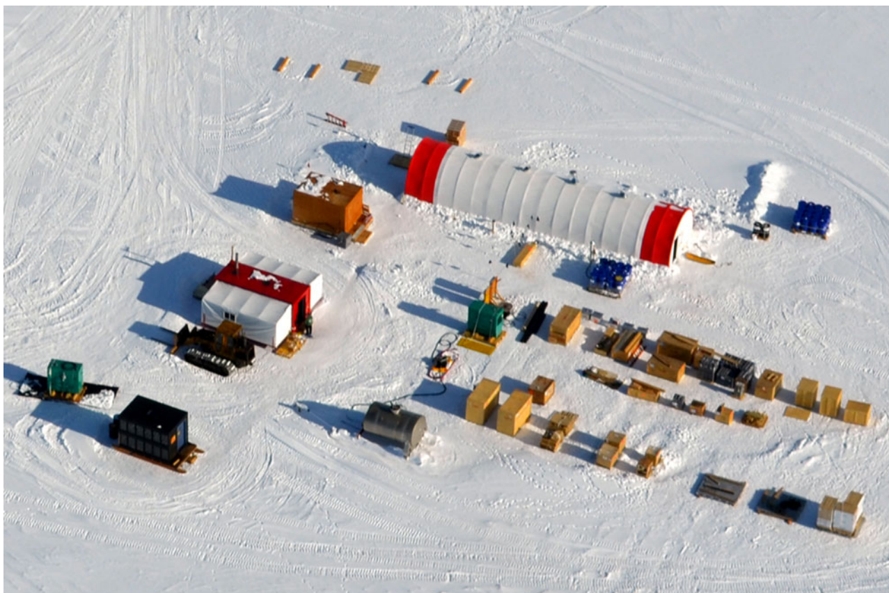
Fig. 2. Aerial view of the drill site showing the four main structures at the site: an outhouse (bottom left corner), a warming hut and mechanical repair space (rectangular white building with red center stripe), a dedicated hut to hang and dry drill fluid-covered clothes (orange rectangular building), and the drill tent (long white and red arch).
