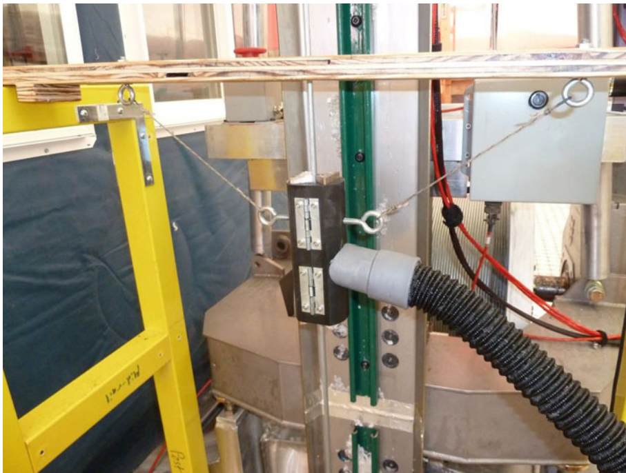
Fig. 8. Cable cleaner with an attached suction hose for removing drilling fluid from the winch cable.
