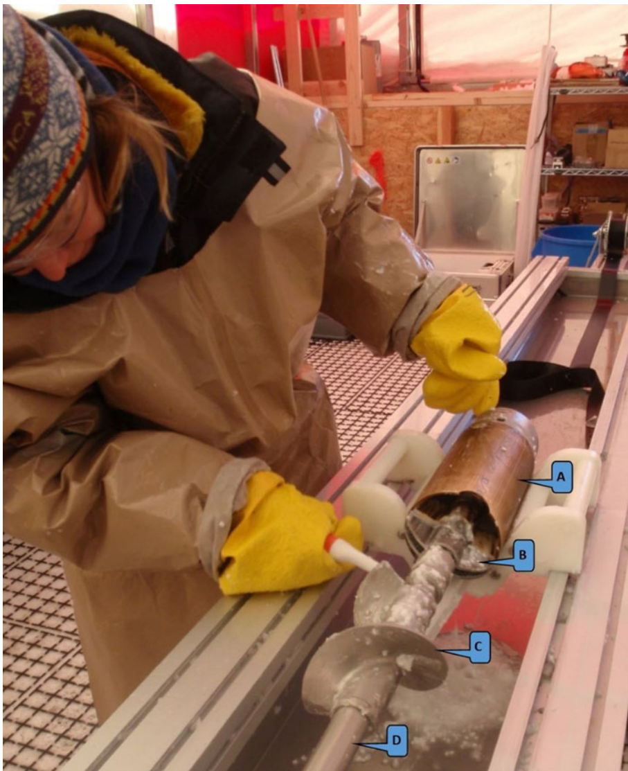
Fig. 12. (a) Chips valve housing with an internal booster. (b) Hinged valve plates. (c) Upper booster. (d) Hollow shaft.
