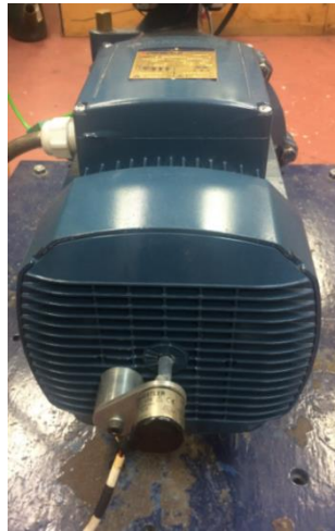
Figure 6-11 Mounted Hengstler shaft encoder
