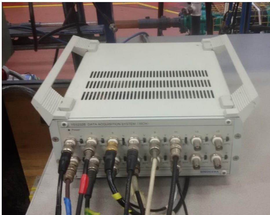
Figure 6-15 YE6232B Data Acquisition System (DAS)
