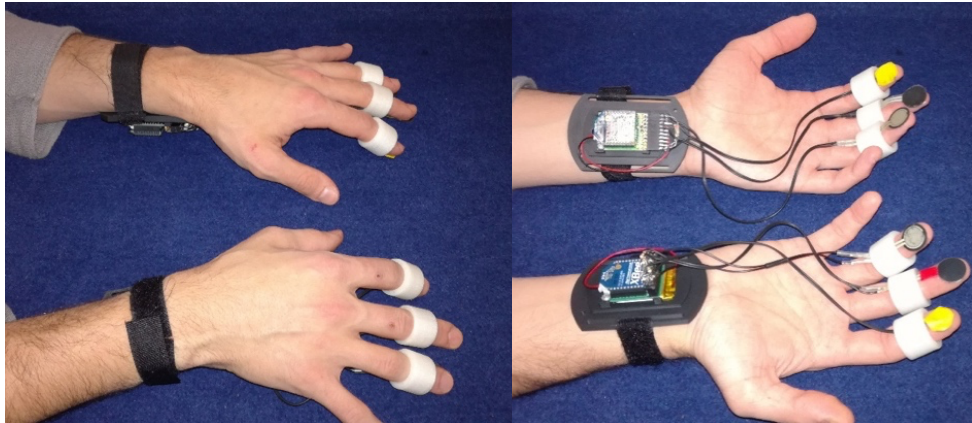
Figure 1. The Piano Hands – MINIBEE and touch sensors, front and palm view (S. Moroz)
