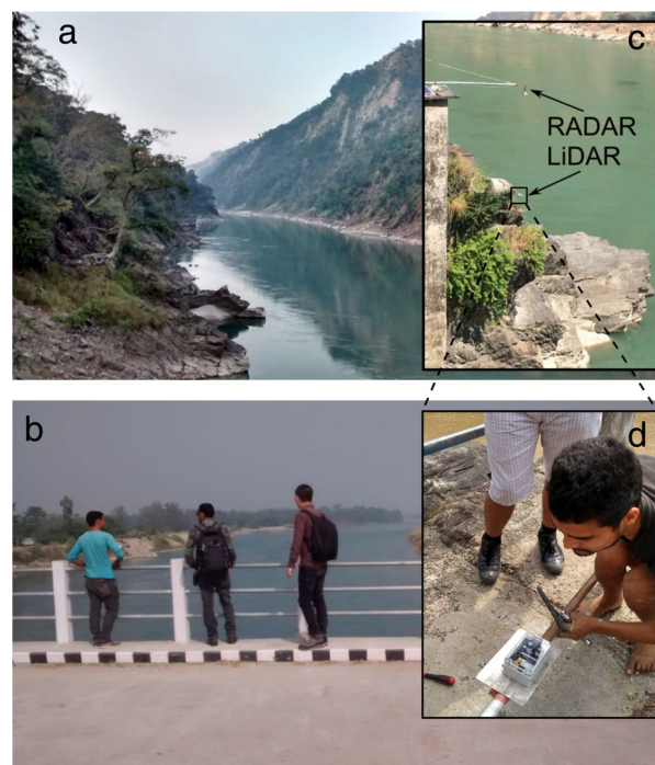
FIGURE 3 (a) Chisapani (upstream) station location, facing north. Note deeply incised river valley. (b) Phanta (downstream) station, looking upstream. Here, the lidar system was clamped to the underside of Sattighat road bridge. See Figure 1 for locations. (c) and (d) Details of lidar sensor and installation on pole at Chisapani. Photographs taken November 2017
