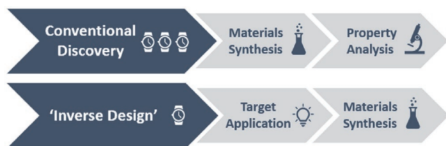
Figure 1. Comparison of conventional materials discovery, where materials are synthesized and then their properties are investigated, to “inverse design” where a material is designed based on a desired target application prior to synthesis. Approximate time cost for each step is indicated (1 clock = quick; 3 clocks = time-intensive).
