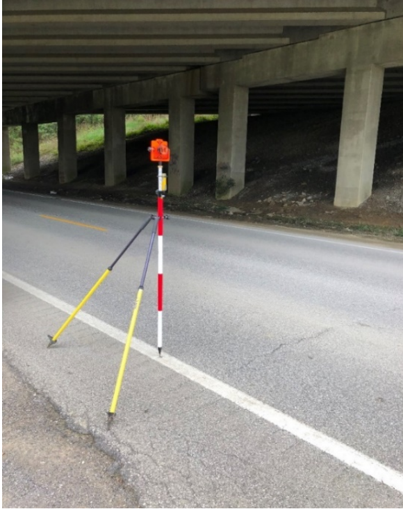
Figure 24. Survey Pole, prism, bipod set up.
