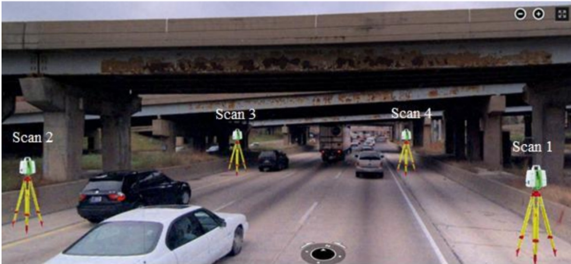
Figure 16. Representation of scan locations. Reprinted from “Applications of Terrestrial laser scanning,” by C. Zhang, D. Ardit, and Z. Chen, 2013, Journal of traffic and Transportation Engineering , 1(5), p. 328.
