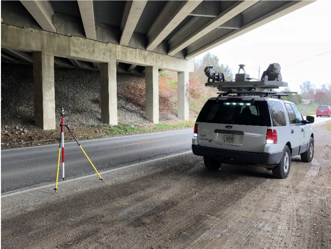
Figure 26. Optech Lynx Mobile Mapping System.
