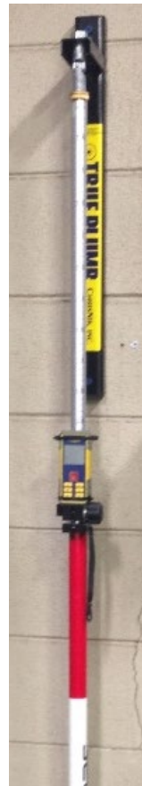
Figure 19. Prism Pole attachment
