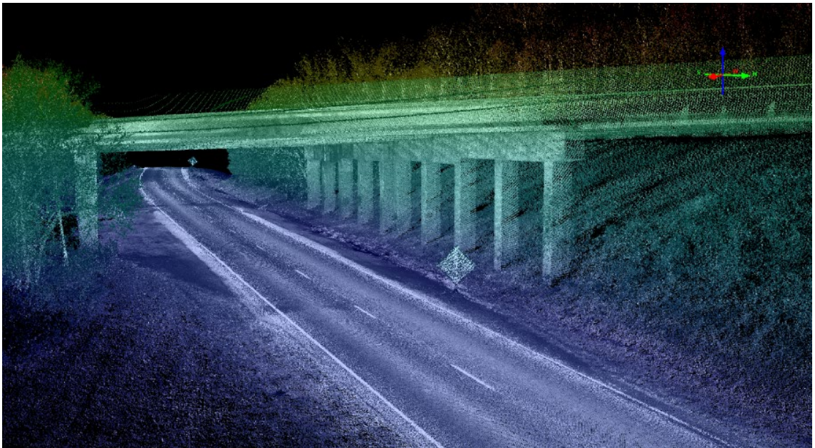
Figure 29. Detected planar surfaces extracted from boresight.
