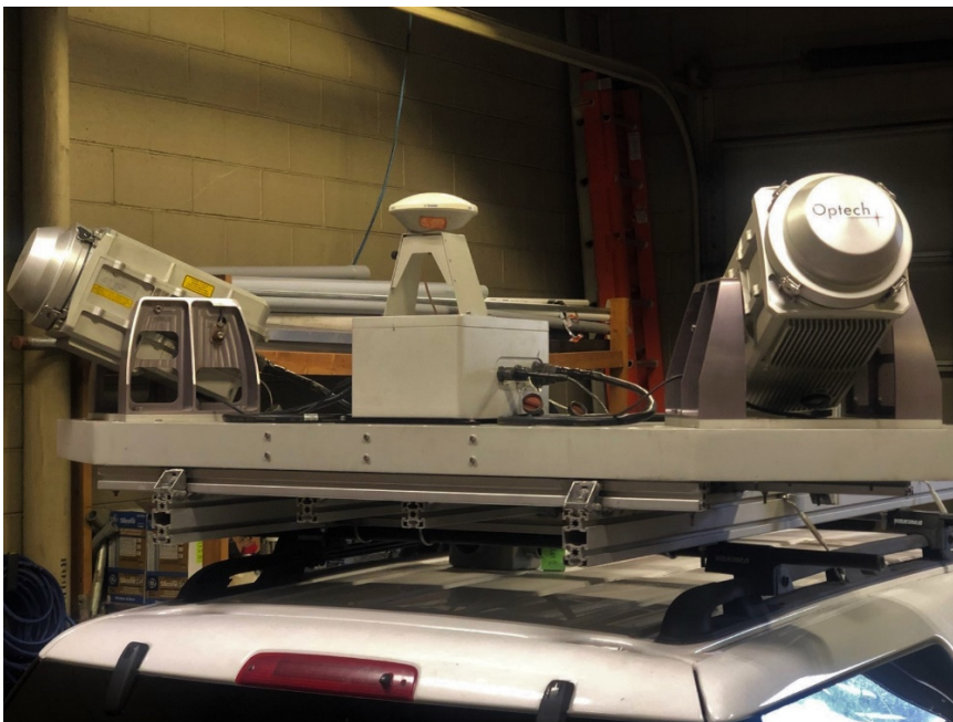
Figure 17. Optech LYNX Mobile Mapping System
