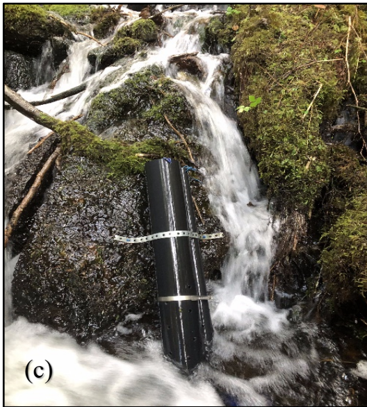
Figure 4.3: Stilling wells at the following study sites: (a) Walkabout Cave resurgence, (b) Walkabout Cave resurgence, and (c) Zina Cave baseflow.
