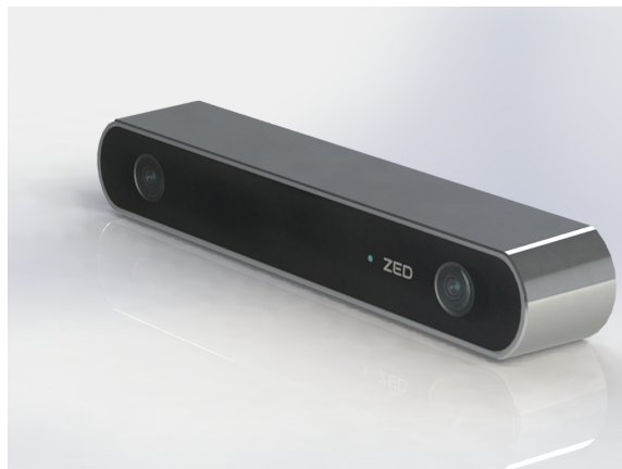
FIGURE A.2: 2K Stereo Camera for Depth Sensing and Spatial AI.
