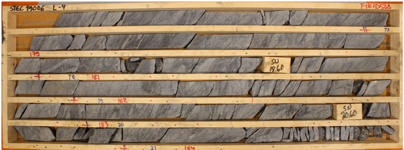
Figure 26: Photos produced using the set-up shown previously. Drill-core box photo can be lined up against the LIBS measurement image to allow for visualisation of element-rich regions, veins, mineral variations etc.
