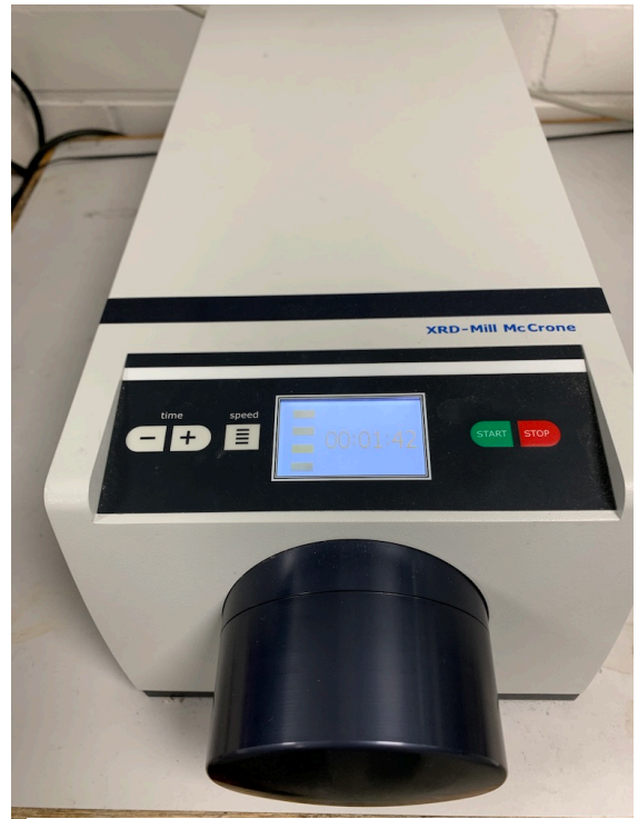
Figure 31: McCrone micronising mill used during this study. Used to reduce the particle size of Kittilä samples and thin disk samples to <5\mu\text{m} in preparation for XRD analysis.
