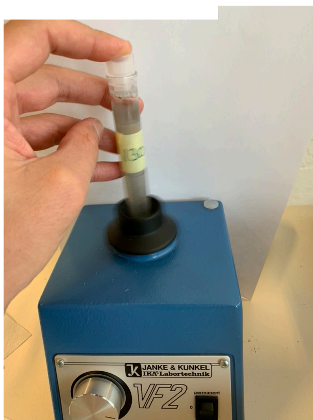
Figure 30: Janke & Kunkel VF2 sample homogeniser used during the sample preparation of TXRF quantitative samples.
