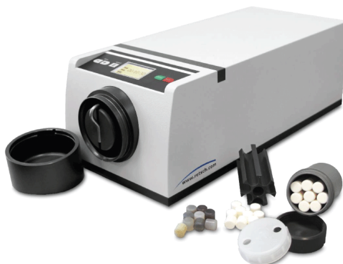
Figure 5: McCrone Micronizing Mill, polypropylene jar and grinding stone selection, including agate which were used to pulverise thin disk and powder samples in preparation for XRD analysis. Image taken from The McCrone Group, 2020.
