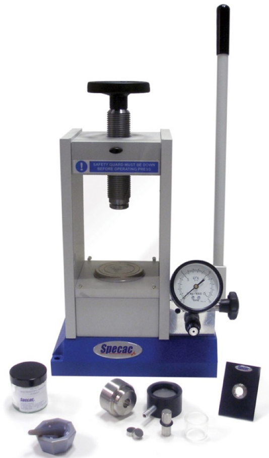
Figure 7: A Specac 15T manual bench-top pellet press and associated die set used to produce pellets for LIBS scanning. Image taken from (Specac, 2020).
