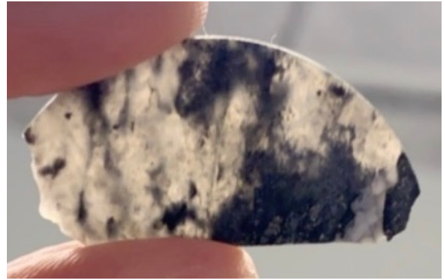
Figure 24: Thin disk sample, approximately 0.2mm thick. Achieved by cutting and grinding. This sample contains quartz veins which have become clearly translucent due to the thickness of the sample. Both sides of the sample display the same structures with the goal of producing LIBS data which is as similar for both sides as possible.
