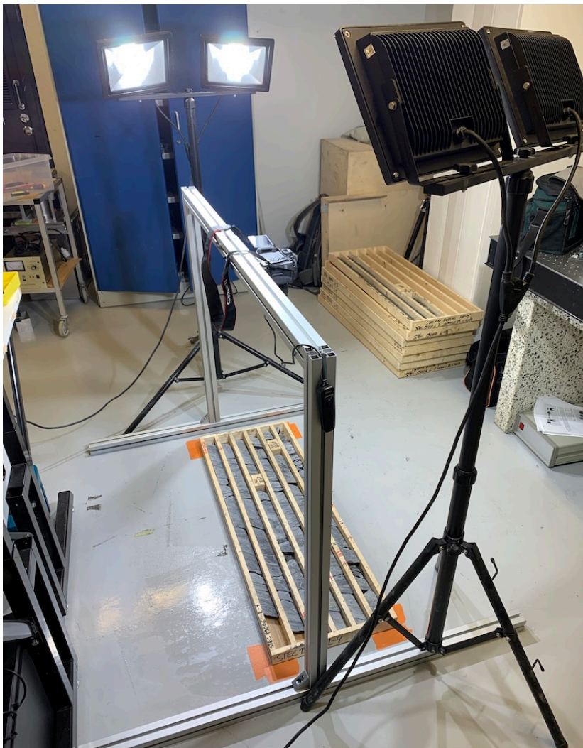
Figure 25: Drill-core box and camera set up to allow for high quality sample images to be made. The images will go into the LIBS software as a comparative feature - photo against LIBS measurement.
