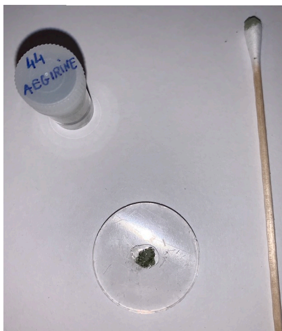
Figure 29: Mineralogical sample 44 (aegirine), previously analysed by XRD, being prepared for semi-quantitative analysis. Q-tip used for transferring sample material onto a sample carrier with a thin layer of silicon grease for adhesion.
