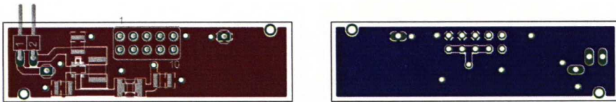
Figure A9: Step-up Converter Module Layout; 1:1 scale
