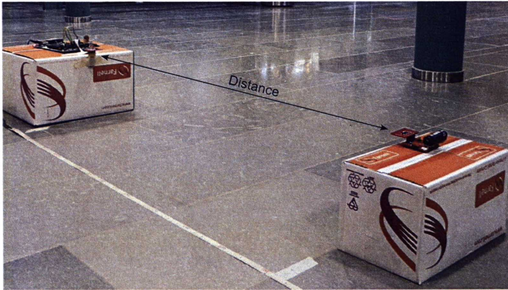
Figure 32: Range Measurement Radio Placement and Orientation
