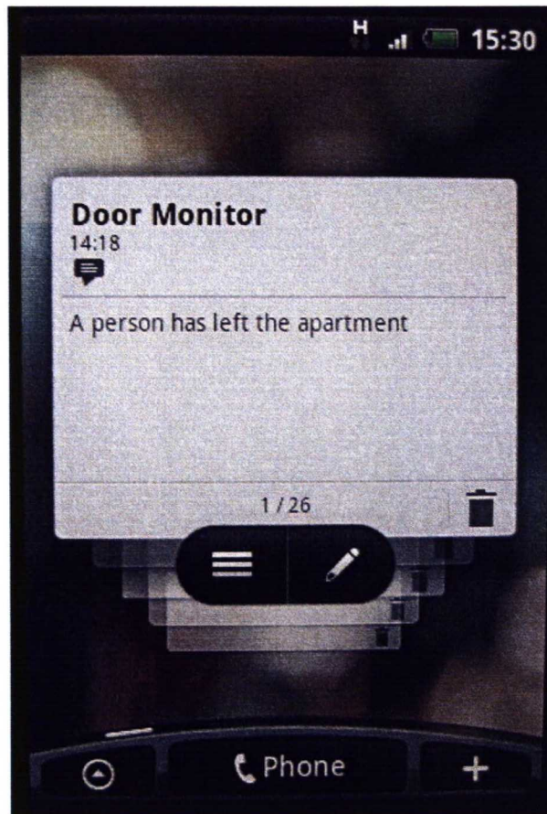
Figure 48: Door Monitor Alarm Message
