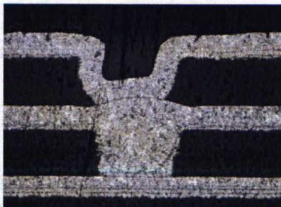
**Figure 1.11:** A SEM image of the cross-section of an overfilled via. The upper layer via has deformed due to the bump on top of the bottom layer via. The created interconnection is unreliable. Picture courtesy of Aspocomp [5].
