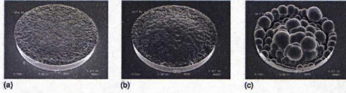
**Figure 1.18:** A SEM image elucidating the effect of mass transfer limitation on plated deposit surface smoothness. The mass transfer conditions are kept constant in every image but plating rate (i.e. deposition current density) is elevated from 5  $\mu\text{m}/\text{min}$  in (a) to 6  $\mu\text{m}/\text{min}$  in (b) and 7  $\mu\text{m}/\text{min}$  in (c).
