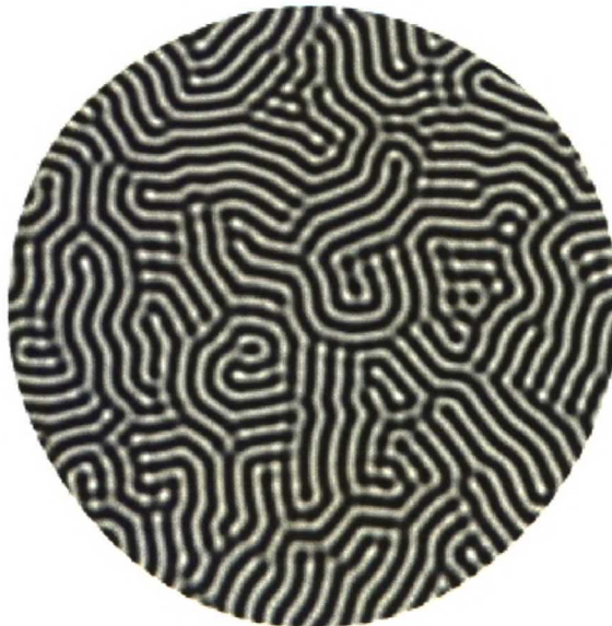
Figure 2.7: Computer simulation of Rayleigh-Bénard convection using the Swift-Hohenberg model. The view is from above. Notice that the convective cells are not ordered as in the ideal situation of Figure 2.6. The dark and light colors denote the domains with upward movement (warmer sparse liquid) and downward movement (cooler dense liquid), respectively. The figure is reproduced from [Karttunen, 2001].
