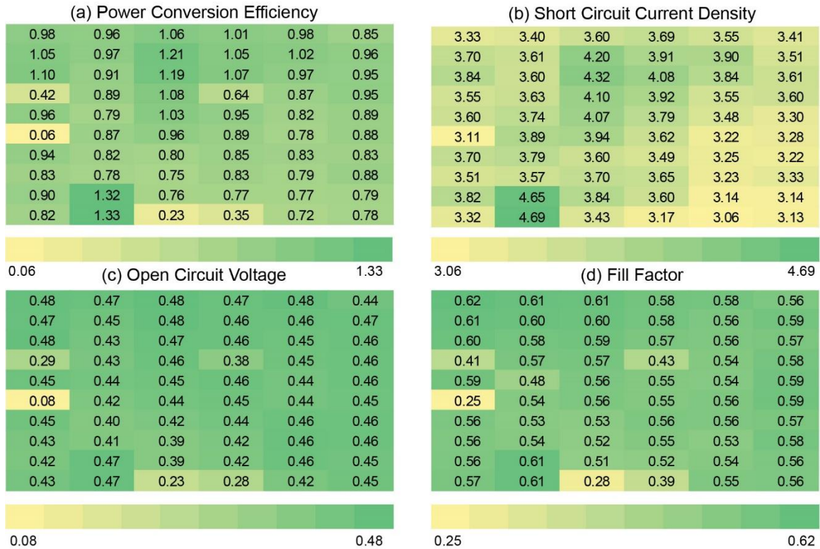
Figure 6.3: Color coded plots showing (a) power conversion efficiency, (b) short circuit current density, (c) open circuit voltage, and (d) fill factor of each pixel device of the CuInSe 2 nanocrystal prototype solar cell shown in figure 6.1 under AM1.5G illumination (100mW/cm 2 )
