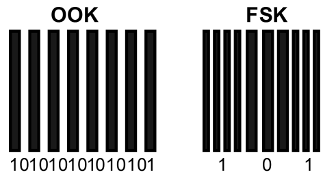
Figure 2.35: OOK and FSK modulation using the rolling shutter effect.
