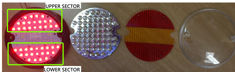
Figure 3.11: Taillight components (from left to the right): PCB with recessed LEDs, plastic mirror, plastic color lens and plastic encapsulation.
