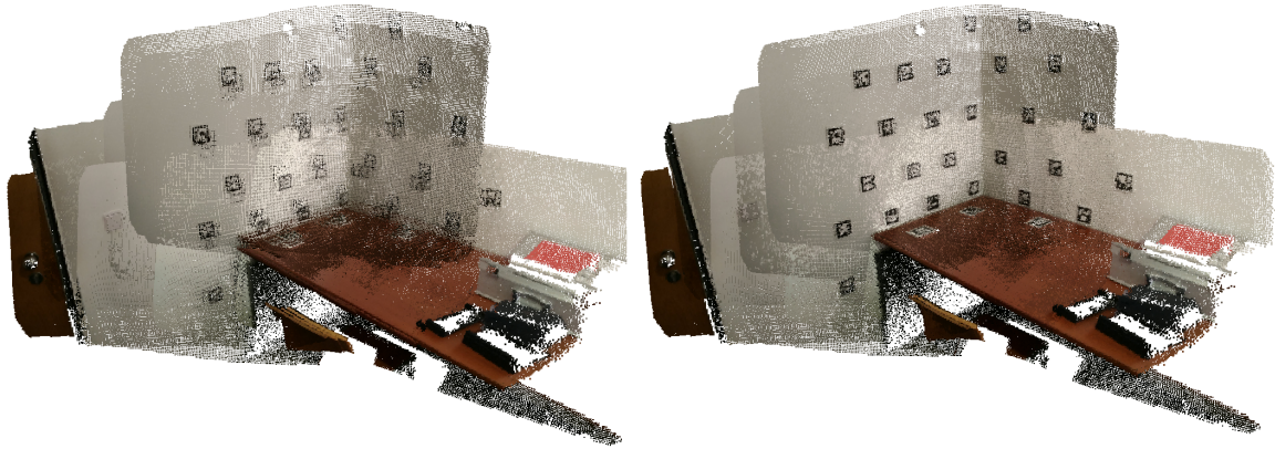
Figure 5.22: Merged point cloud coloured with texture obtained from images. Before optimization on the left and after optimization on the right (meshlab).
