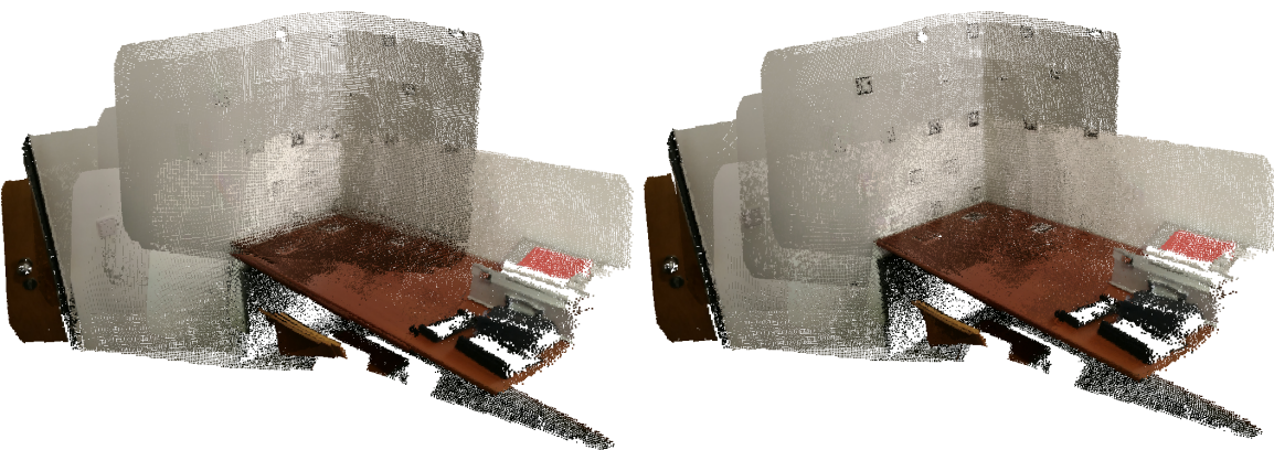
Figure 5.21: Point cloud coloured with texture obtained from restored images, no cross-inpainting. Before optimization on the left and after optimization on the right (meshlab).
