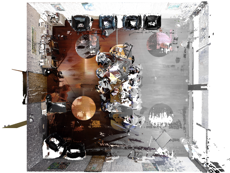
Figure 6.1: FARO generated point cloud after downsampling.
