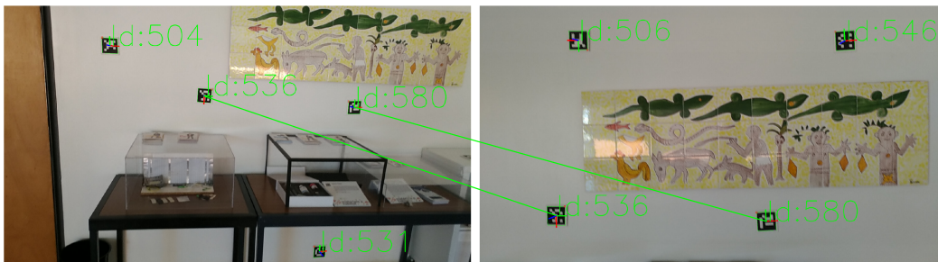
Figure 2.6: Representation of detection and matching of aruco markers for a pair of captures.
