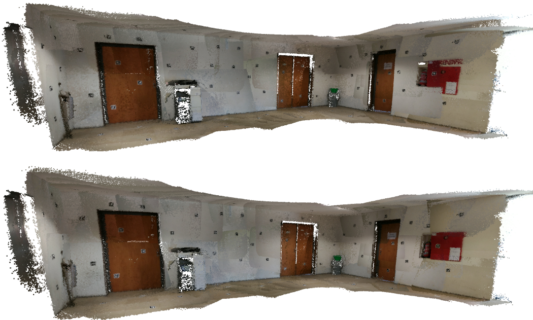
Figure 6.9: Lobby dataset coloured with texture obtained from original images. Before optimization on the top and after optimization on the bottom.
