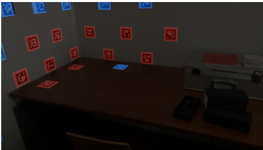
Figure 5.17: Final mask after optimization. Masks obtained from aruco marker detection in red and masks obtained from projections from other cameras (Cross-Inpainting) in blue.
