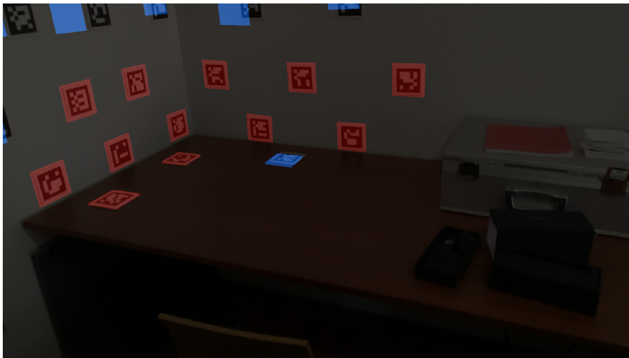
Figure 5.16: Final mask before optimization. Masks obtained from aruco marker detection in red and masks obtained from projections from other cameras (Cross-Inpainting) in blue.
