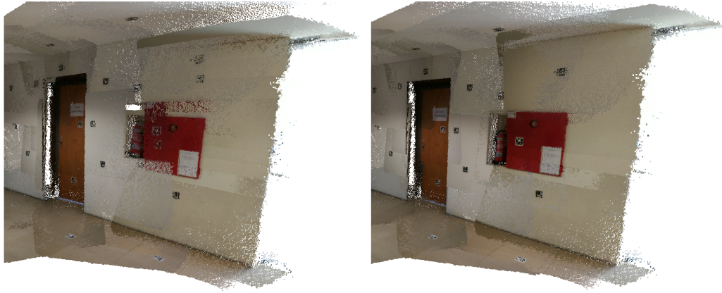
Figure 6.10: Lobby dataset coloured with texture obtained from original images (detail). Before optimization on the left and after optimization on the right.
