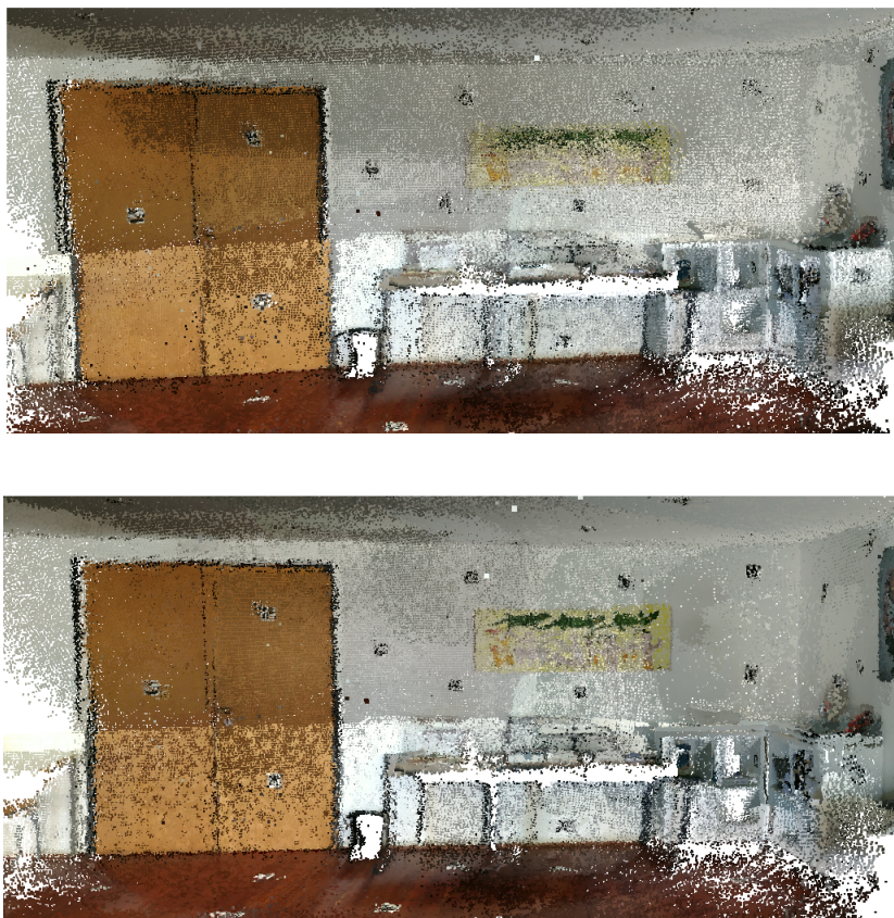
Figure 6.5: MeetingRoom dataset coloured with texture obtained from original images (detail 2). Before optimization on the top and after optimization on the bottom.
