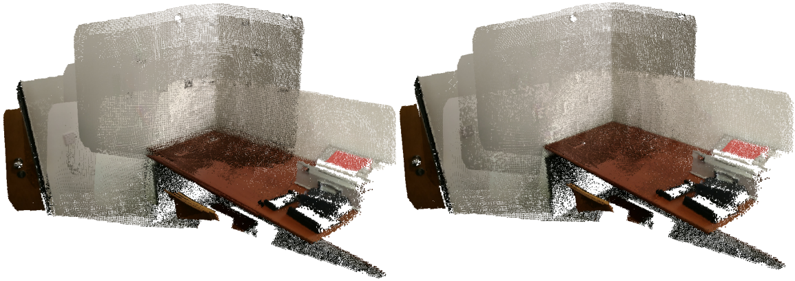
Figure 5.20: Point cloud coloured with texture obtained from restored images, using cross-inpainting. Before optimization on the left and after optimization on the right (meshlab).
