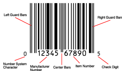
Figure 1.1: Brief explanation of the numeric values often displayed under a barcode tag. [6]
