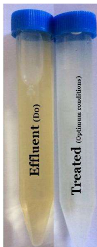
Fig. 5.2. 4. Effluents before treatment with nanomaterials (left) and the sample of the treated effluents under optimum conditions (right).
