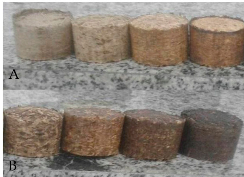
Figure 1. Briquettes produced at 10.34 MPa pressure. (A) = Briquettes produced from fresh biomass, left to right: bagasse, coffee, eucalyptus, and pine. (B) = Briquettes produced from torrefied biomass, from left to right: coffee, eucalyptus, pine, and sugarcane bagasse.
