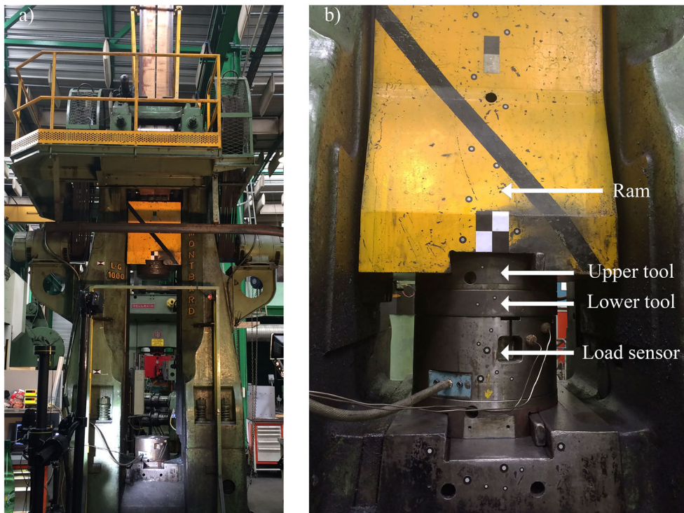
Fig. 1 a Global view of the machine. b Tools and sensor used for the experimental protocol
