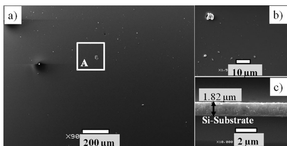
Figure 2. SEM images of the as-deposited ZrN-01 coating on Si substrate: (a) global view of the surface, (b) magnified image of the region enclosed by the white square (area A) and (c) cross-section image of the same sample.
