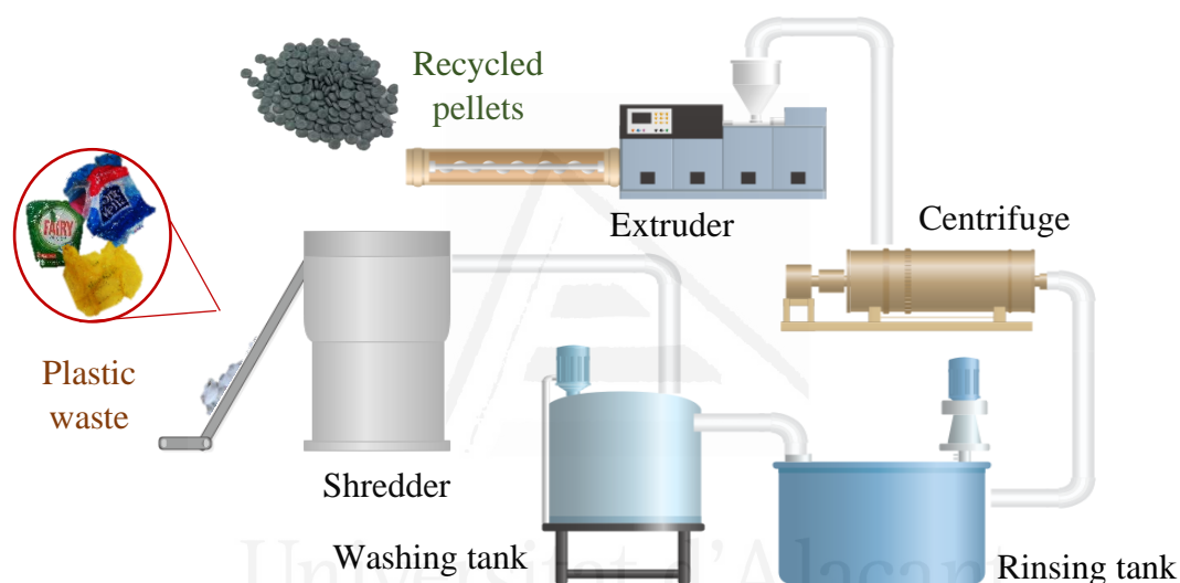
Figure 1.5. Simplified diagram of a conventional mechanical recycling process. Source: own elaboration (made with Edraw Max).
