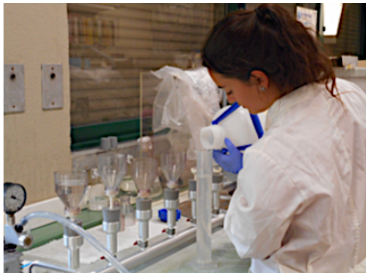
Figure 4.2 - Water sample filtering procedure.
