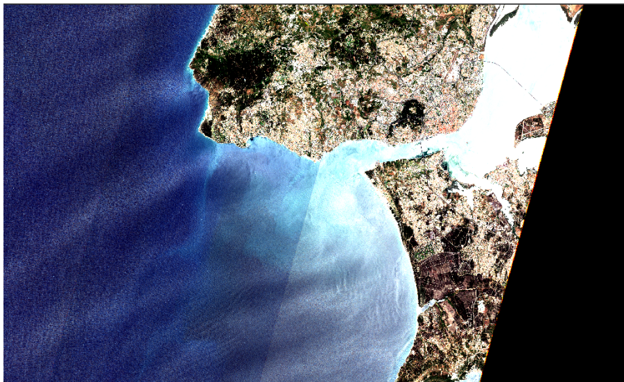
Figure 6.8 - Example of RGB S2-B image contaminated by a strong sun-glint. On the right, the Tagus estuary is completely covered by the reflection of sun which masks the water features. RGB image captured by S2-B satellite on the 28-05-2019.
