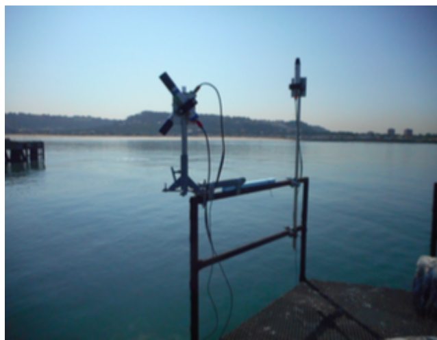
Figure 4.4 - TriOS/RAMSES hyperspectral radiometers as installed on the pontoon rail.
