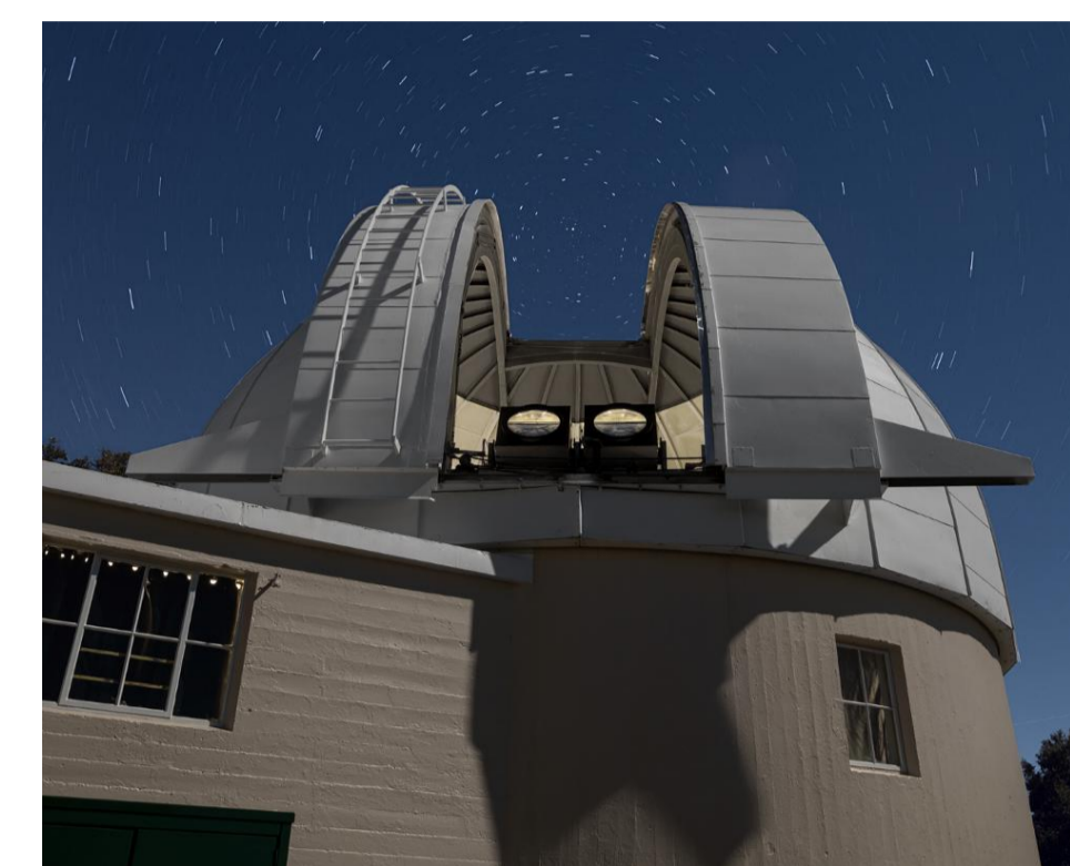
Figure 2: two side-by-side PANOSSETI telescopes pointing in the same direction have been deployed inside the Astrograph dome at Lick Observatory (photo courtesy: Laurie Hatch Photography).
