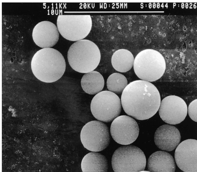
Figure 1. The particles used for instillation in human subjects were smooth and spherical with a count median diameter of 2.6 \mu\text{m} and geometric standard deviation ( \sigma_g ) of 1.3. The particles were generated from colloidal \text{Fe}_2\text{O}_3 made from the hydrolysis of \text{FeCl}_3 . Bar in the top margin of the photograph = 10 \mu\text{m} .
