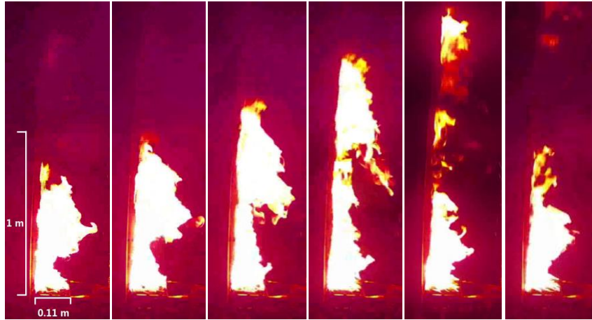
160 Fig. 3 Sequential flame images taken from the side of a rectangular fire located against a CS board at 161 time intervals of 0.08 s ( R = 7.45 , \dot{Q} = 84.8 kW)
