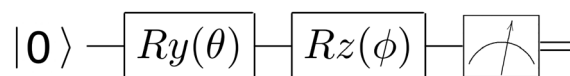
Fig. 1 Mean-field circuit acting on a single qubit has been employed to determine the lowest bands of silicon. It consists of a polar rotation ( R_y ) followed by an azimuthal rotation ( R_z ). In last step, the expectation value of \hat{H}_k is measured.
