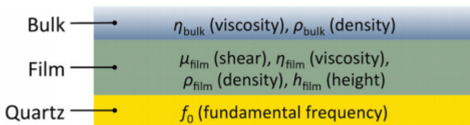
Figure 1.8 Schematic representation of Voigt based viscoelastic film model, with a viscoelastic film on a quartz in contact with a Newtonian bulk liquid labeled with the seven physical parameters that fully define the system (McNamara and Blanford, 2016)
