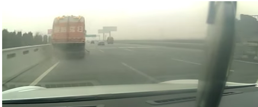
Figure 2-2: Tesla Vehicle not Identifying the Truck Ahead and Resulting in a Collision (Lambert, 2016)
