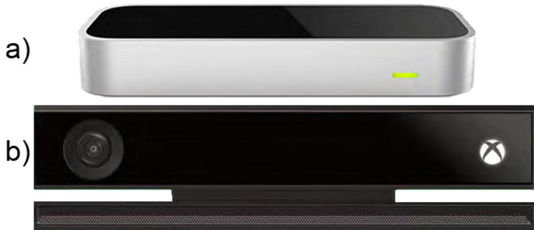
Figure 2.6 - Two prominent optical tracking sensors; a) Leap Motion (Motion, 2013), b) Kinect (Microsoft, 2014)
