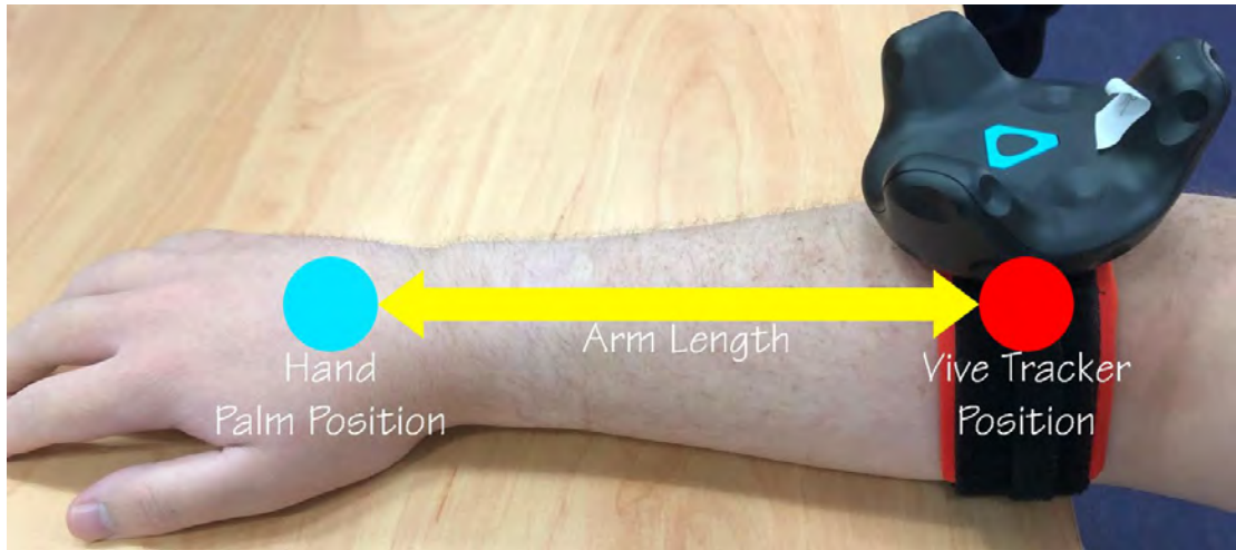
Figure 3.19 – HTC Vive Tracker mounted onto a user’s arm using the Manus Vive Tracker arm mounts
