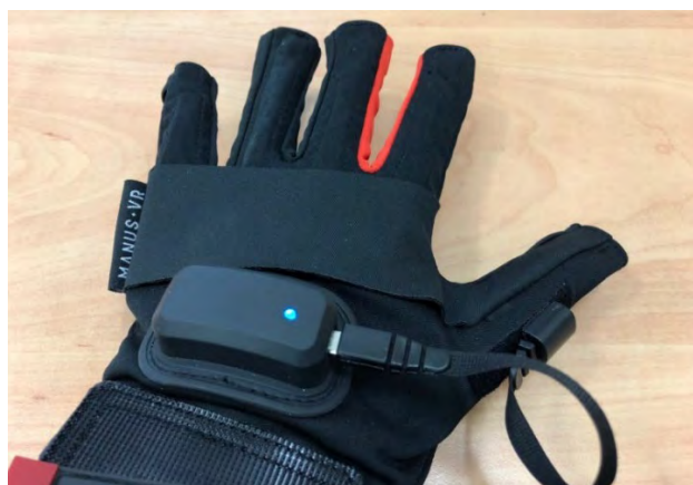
Figure 0.9 - Photo of the Manus VR glove, with the hand in an open hand pose.
