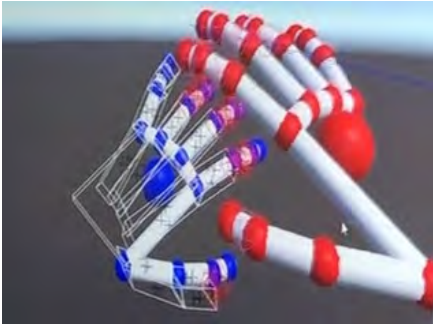
Figure 5.11 - Custom Cube-based Geometry generated around the virtual hand's bones and palm
