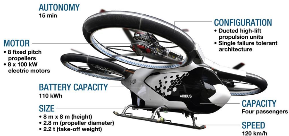
Figure 8: CityAirbus technical data [22]
