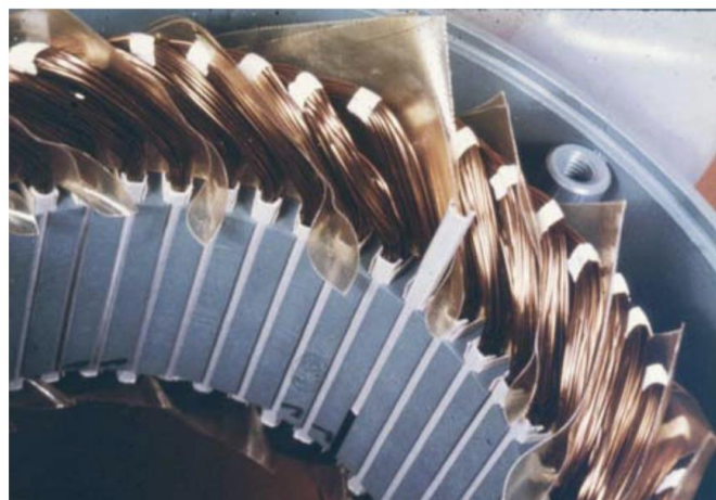
Figure 24: Slot wedges and phase insulation seen with the winding in place; one wedge is partially inserted [43]
