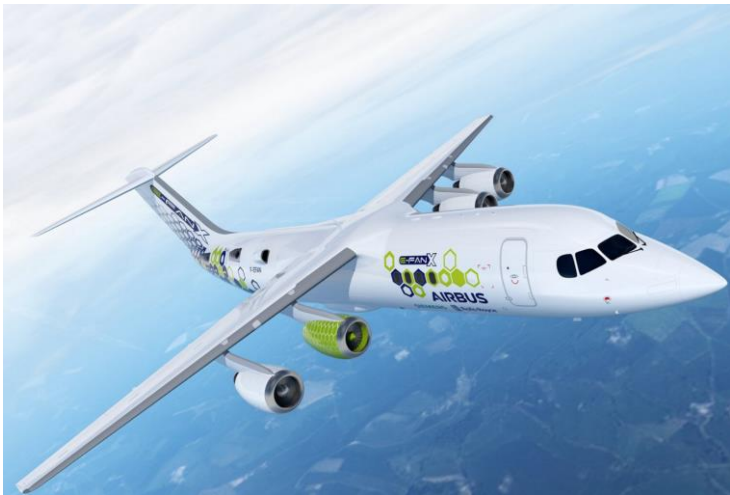
Figure 7: Airbus-Rolls Royce E-FanX (in green : the electric propeller) [21]
