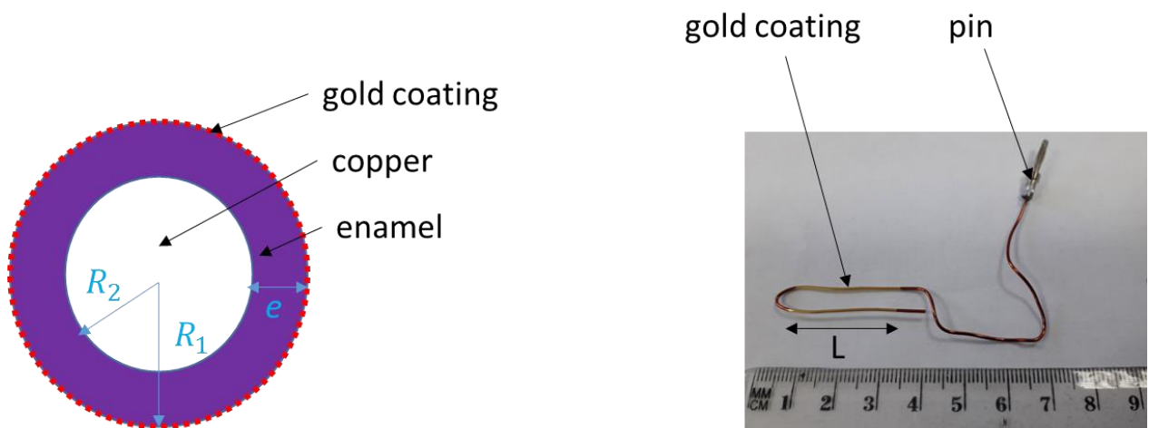
Figure 105: Gold metallization of an enamelled copper wire. Left) Equivalent 2D-coaxial capacitor - R_1 : external radius; R_2 : copper radius; e : enamel whole thickness; Right) Real sample for test in the Novocontrol.
