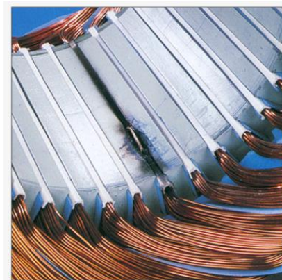
Figure 53: Consequences of PD on a stator winding insulation; left) Corroded enamel layer [40]; right) Slot liner flashover [74]
